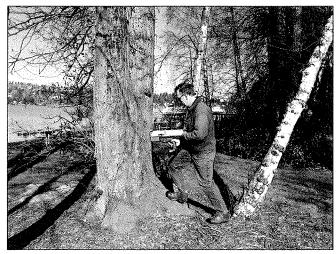
In the primary examination of the root crown and trunk a mallet is used to test for loose bark. Bark lifting can indicate dead or hollow areas and give signs of the presence of decay in the root crown zone and at the base of the trunk. The mallet may be used to "sound" for decay but
