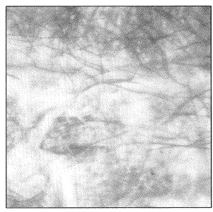
is known as setal hyphae and is a fungal structure which shows that *Phellinus* weirii is present. Extensive de-lamination of wood tissues and decay are to be expected where setae are present.
